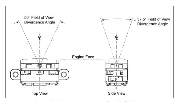
Figure 27. Field of View, Divergence Angle (model IS4910-01 shown)
